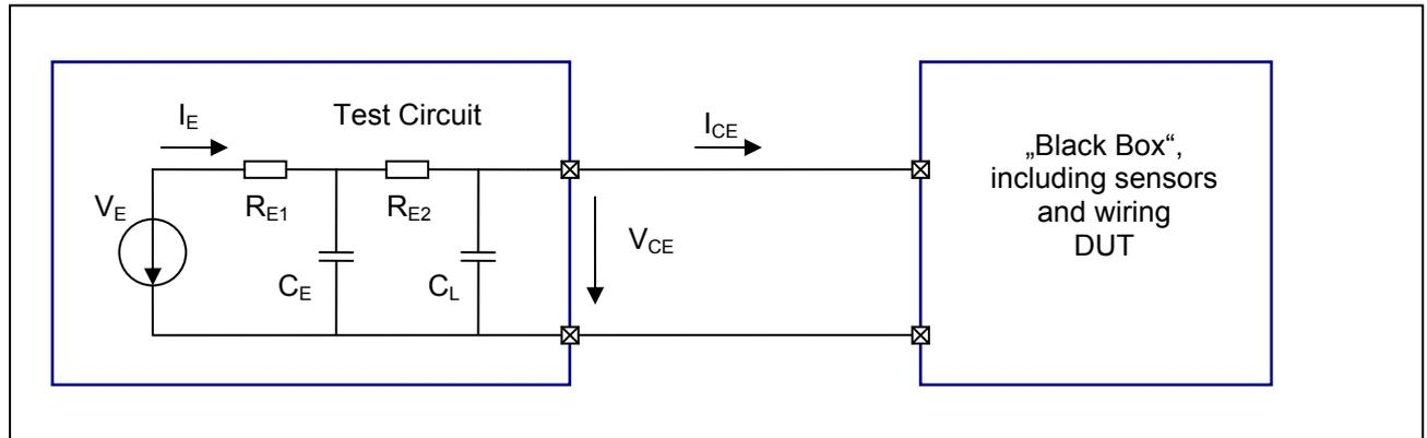
Figure 38 Reference test bench for bus testing
