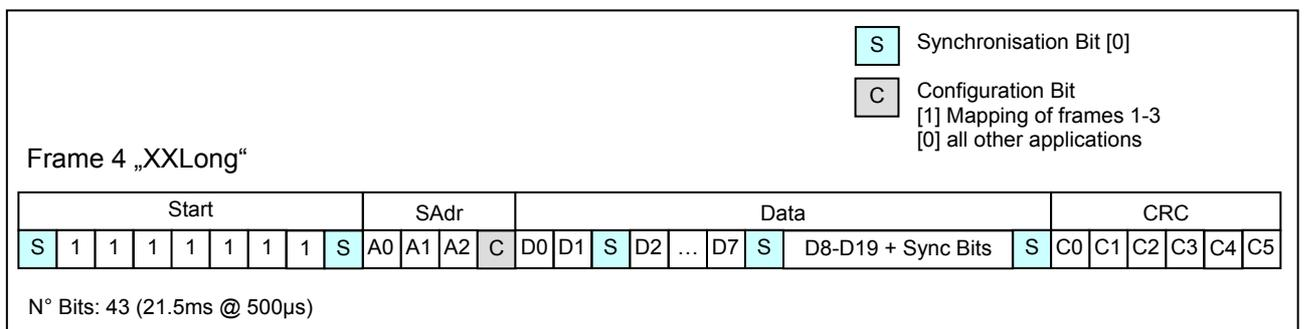
Figure 25 Data frame4 ECU to Sensor Communication
