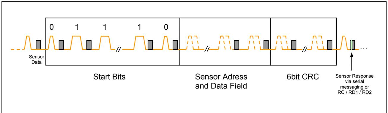
Figure 24 Data frame ECU to Sensor Communication –e.g. Pulse width method with frame format 4 (frame formats 1-3 are also applicable)
