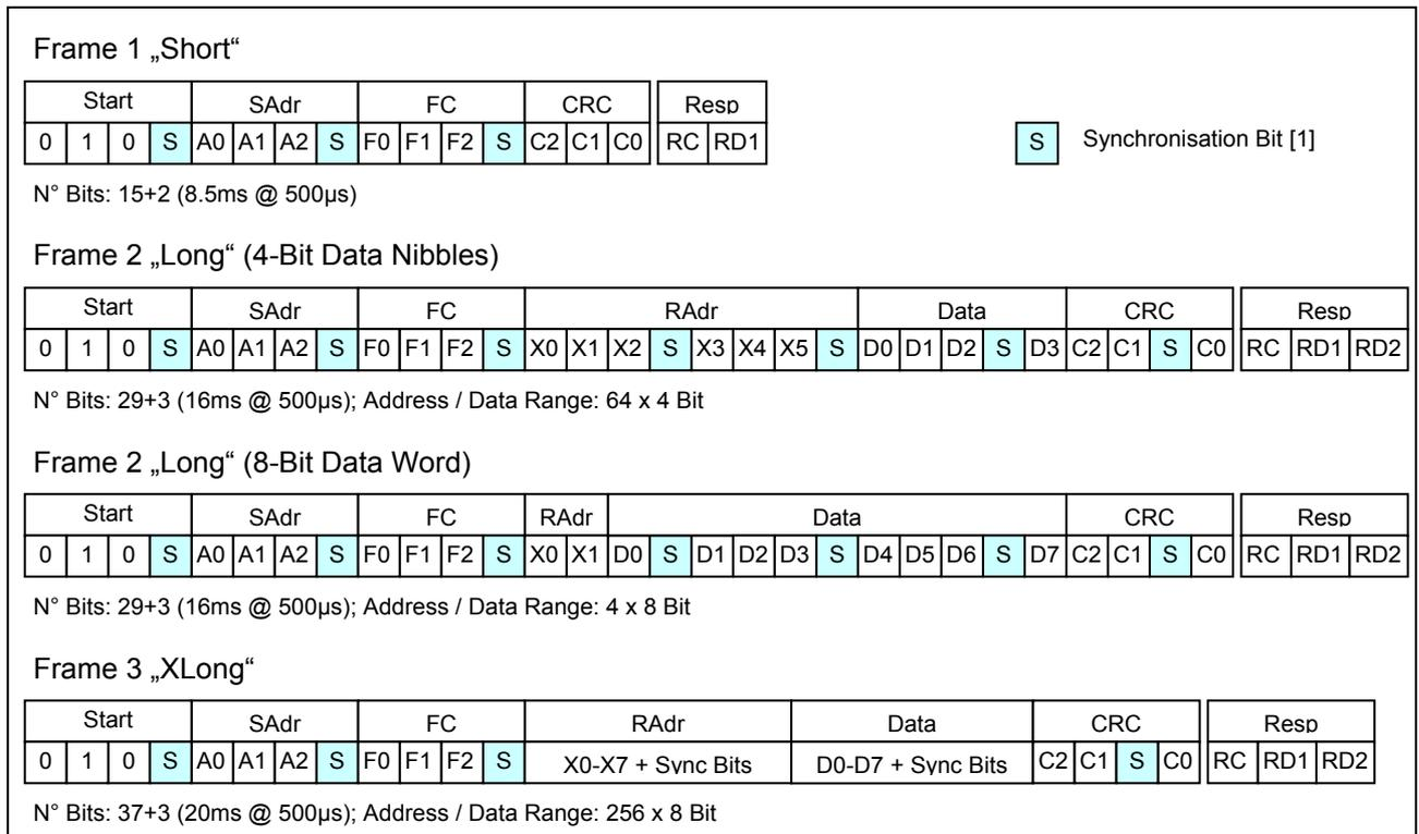
Figure 23 Data frames 1-3 ECU to Sensor Communication
