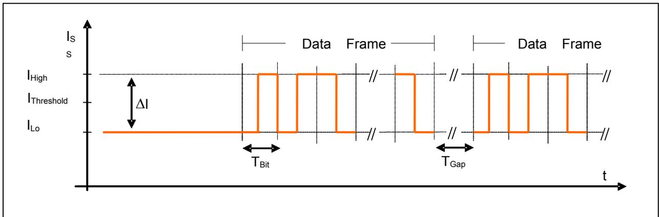
Figure 31 Data Frame Timing
