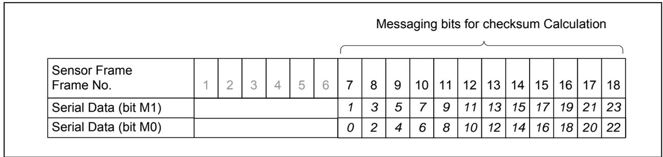
Figure 19 Read in order for checksum generation
