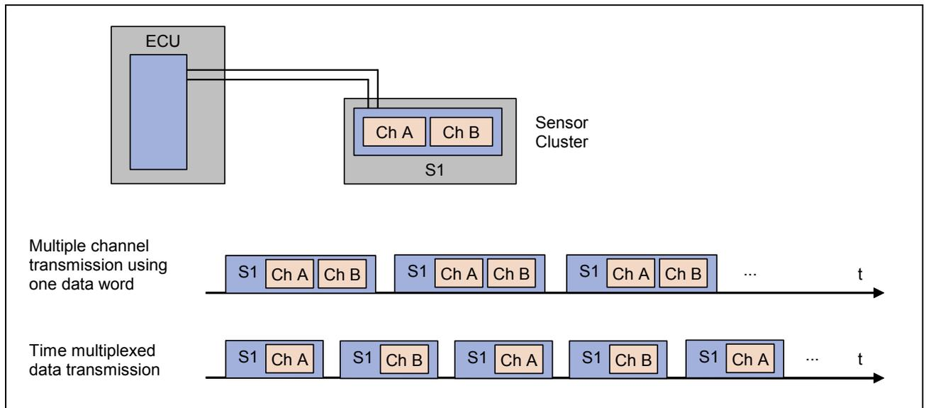
Figure 12 Implementation example sensor cluster
