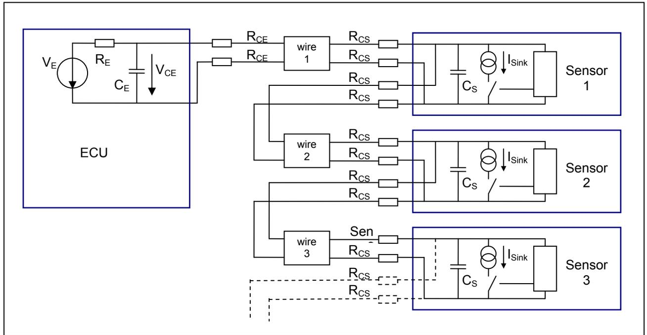
Figure 10 Example for a pass-through configuration (simplified schematic)
