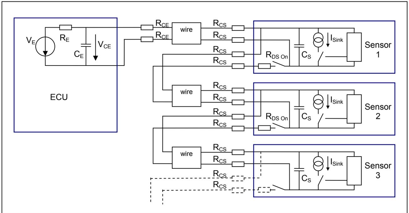
Figure 11 Synchronous Daisy Chain Bus (simplified schematic)
