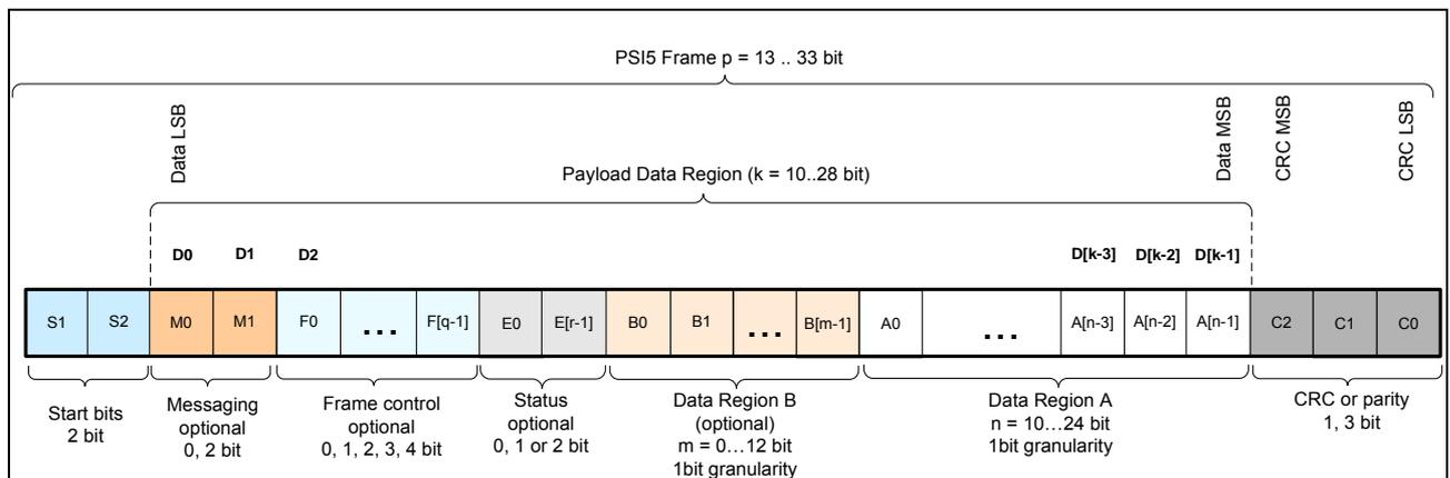
Figure 16 different parts of the PSI5 data frame
