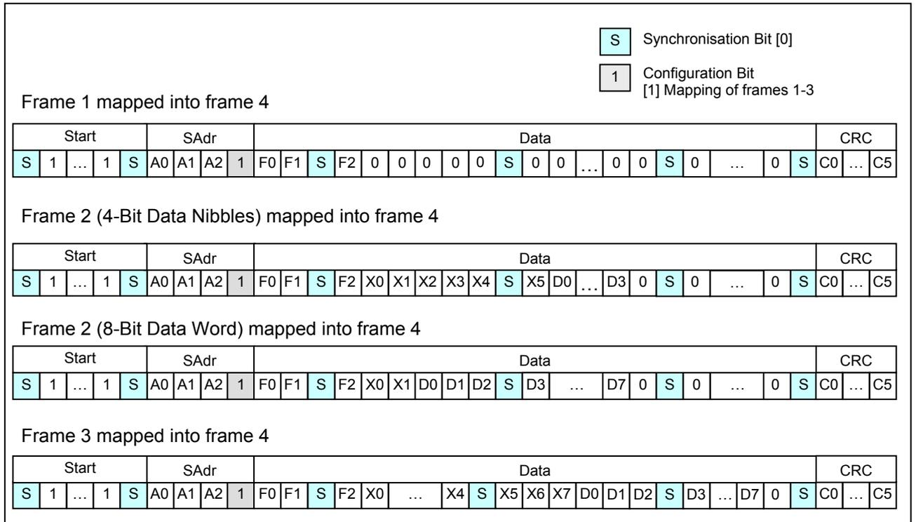
Figure 26 Mapping of frames 1-3 into frame 4
