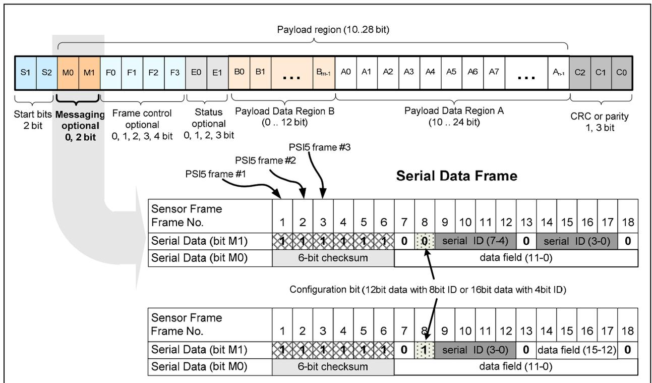
Figure 18 Serial Data Frame generated by the two messaging bits of the sensor data frame (messaging channel)
