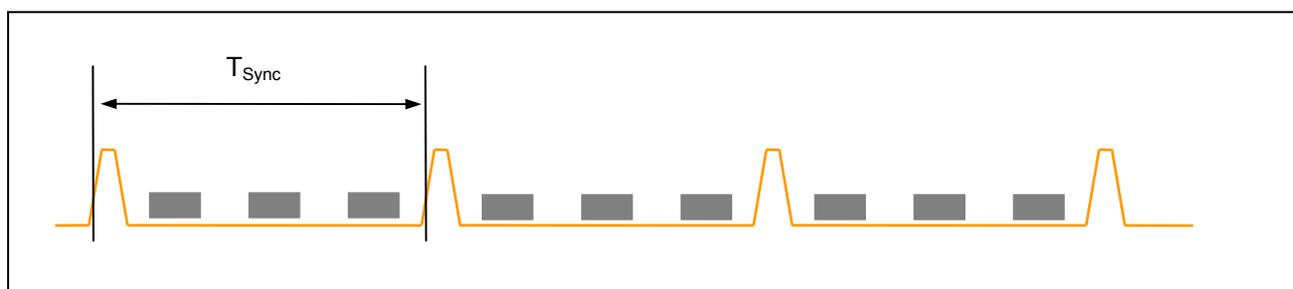
Figure 5 Fixed time triggered synchronous operation
