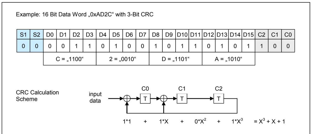
Figure 15 16 Bit Data word example with 3-Bit CRC
