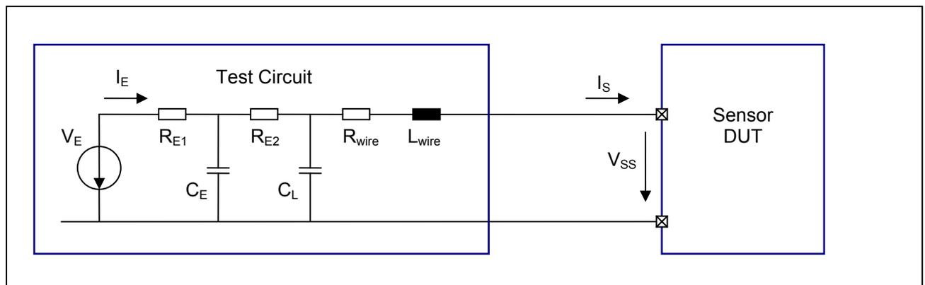
Figure 36 Reference test bench for sensor testing
