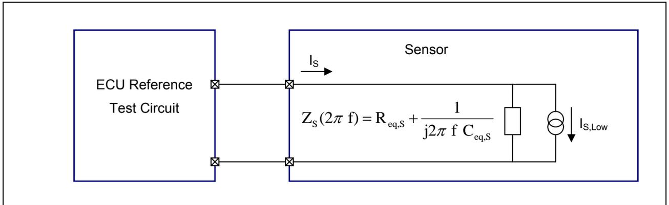
Figure 37 Reference circuit for sensor damping behaviour
