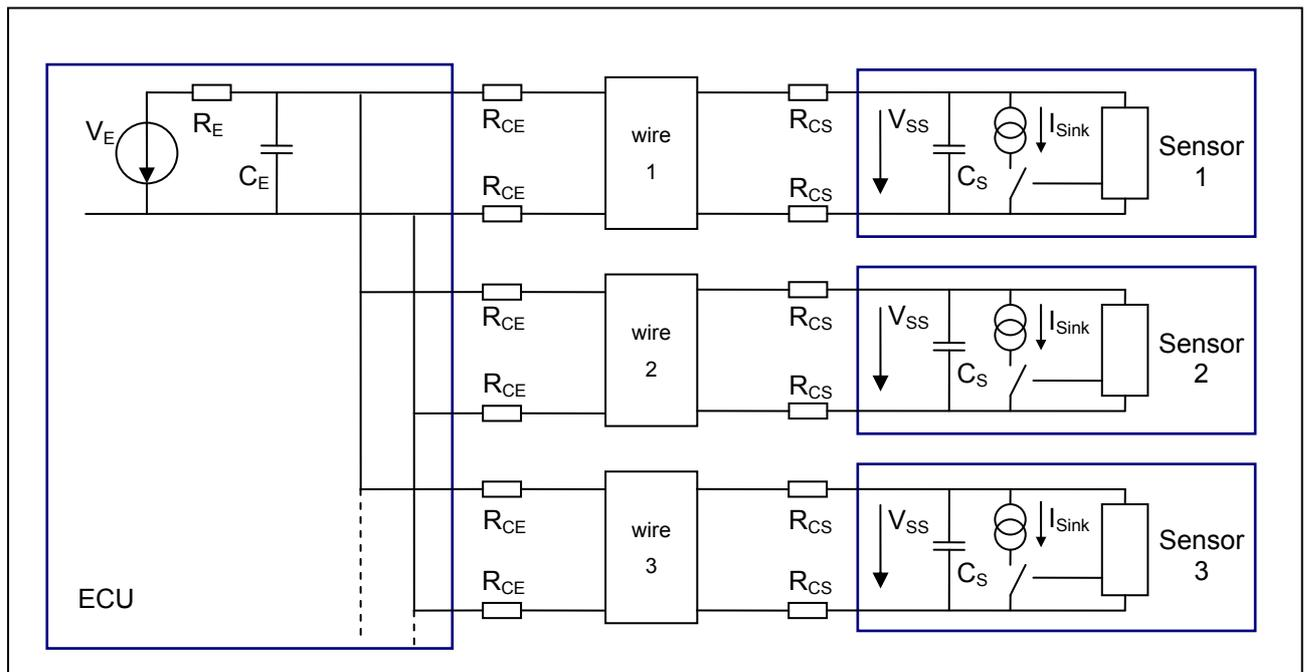
Figure 9 Synchronous Parallel Bus Mode (simplified schematic)
