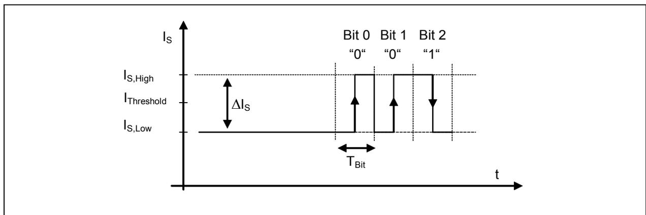
Figure 13 Bit encoding using supply current modulation
