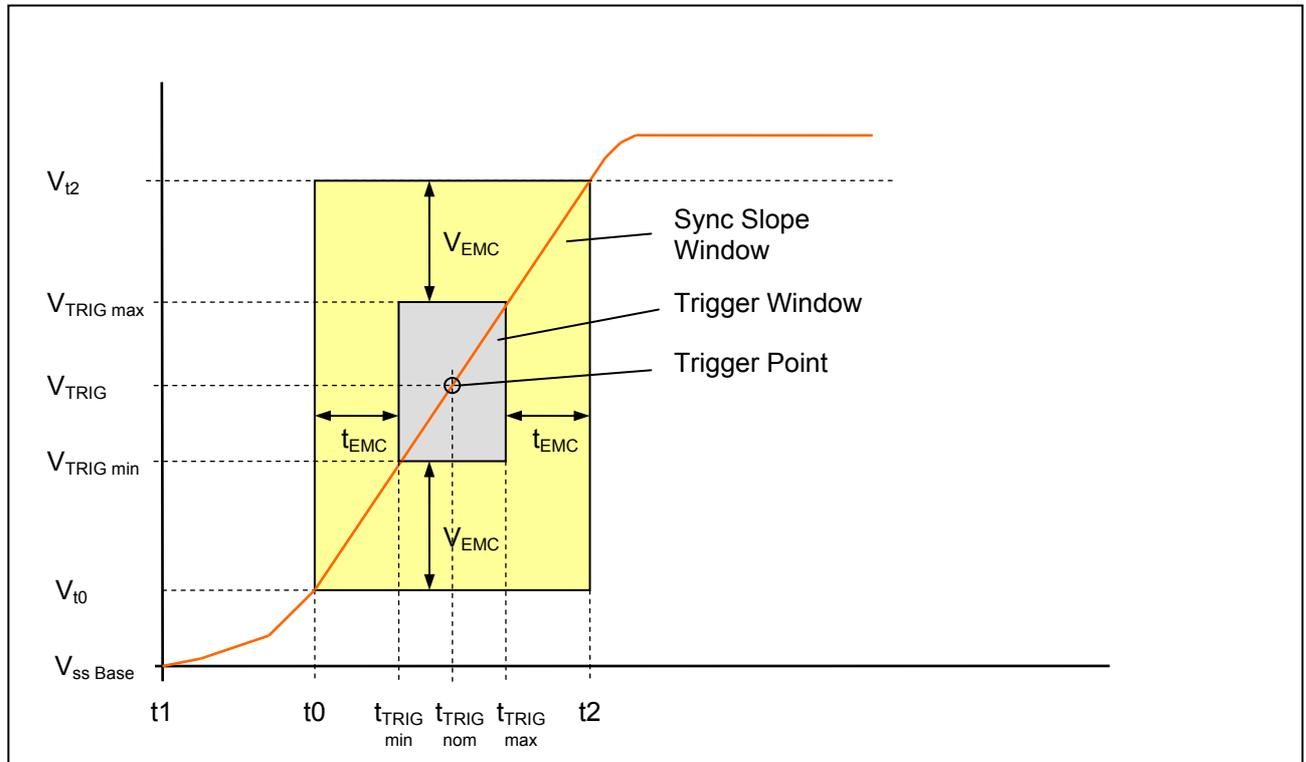
Figure 33 Synchronization signal detection in the sensor
