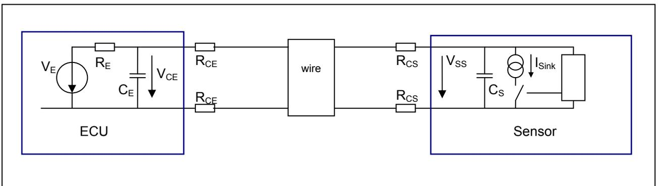
Figure 4 Single sensor configuration (simplified diagram)
