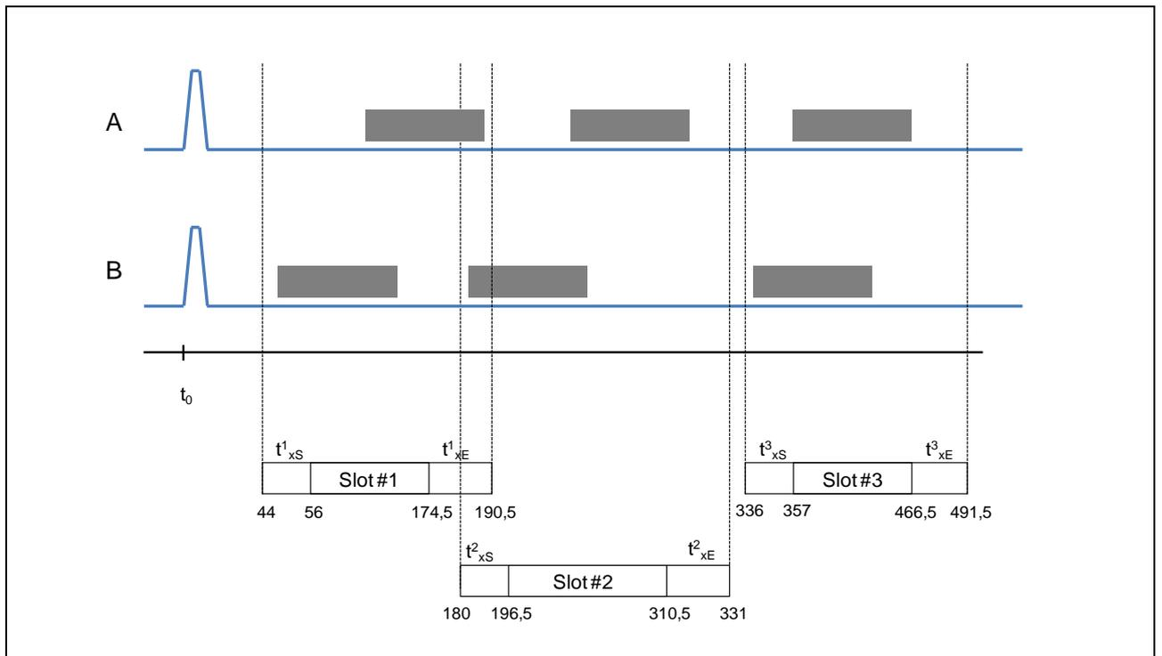
121 *Figure 3 Possible message timing for overlapping slot timings*
